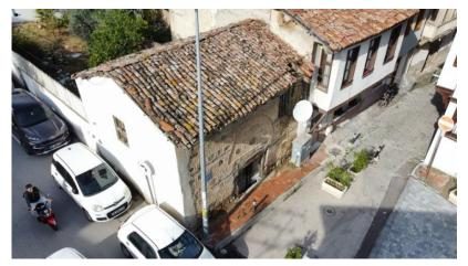
A part of the building from the late Ottoman period extending to İpar Street was used as a winery in previous periods, but it was demolished during the street widening works. The wall of the building facing the street is made of rubble stone. The upper parts of the bricks were oversailed with red paint. The facade wall was masoned with perforated bricks and plastered with mortar. It has a wooden double-winged door framed by a round brick arch.
